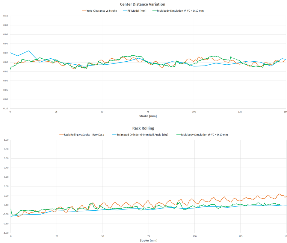
Figure 17 Gear set 1 – rack rolling [mm] and yoke clearance [deg] test: experimental data (orange), multibody simulation (green), analytical estimation (blue) (see online version for colours)
